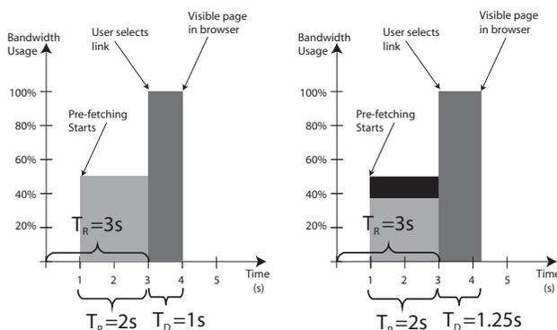
Fig. 3. Browsing with optimal (left) and non-optimal (right) low-bandwidth predictive retrieval
